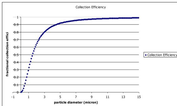
Collection efficiency increases with particle diameter. We expect  $d_{50} = 1.4$  microns for our cyclone.
