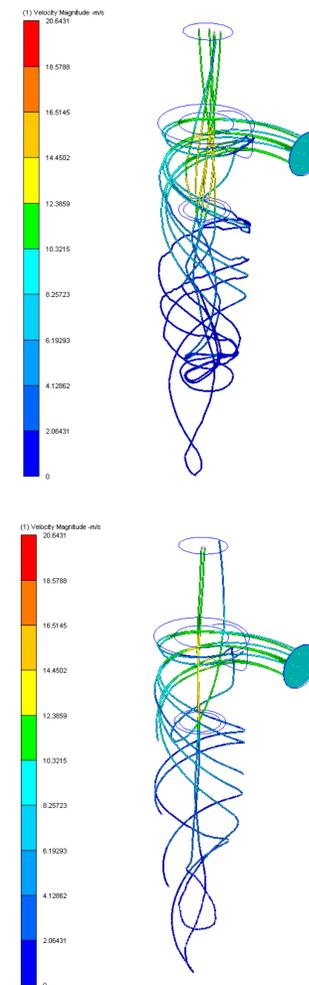
We used particle traces to observe the air flow and particle behavior in the cyclone. Shown above are massless air traces (top), in which all traces escape to the outlet; and 0.5 micron massed traces (bottom), in which some particles escape, and the others are trapped on the cyclone wall.
