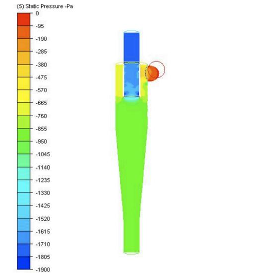
Our simulations reproduce the experimentally observed pressure drop across the cyclone. Increased pressure drop is the trade-off for increased collection efficiency. The static pressure drop across the cyclone is approximately 900 Pa in good agreement with our experimental results.
